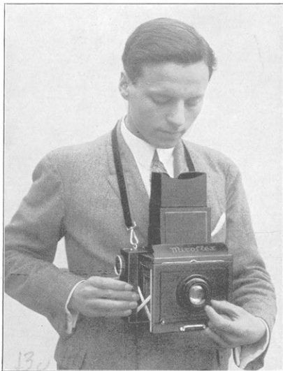
Fig. 4 Fine focussing and exposure whilst watching the picture
